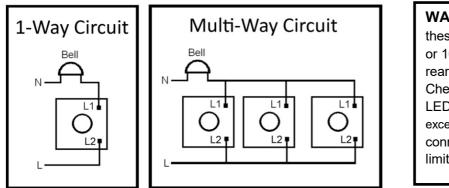
**WARNING:** The switches in these products are rated at 6 or 10A (Please check the rear of the product for rating). Check the in-rush current for LED bulbs or drivers does not exceed 6 or 10A before connecting. Fit inrush current limiters where necessary.
